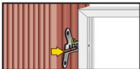
Hang ProtectFIX on the window frame screw FBS-Z from the inside or outside. Position the screw in one of the four grooves and align the ProtectFIX horizontally.
