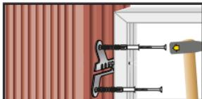
Secure ProtectFIX with two CELO multifunction frame plugs MFR SB 10-80 TX in the base material.
